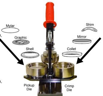
Note: You must use a shim that you have bent.(As pictured here) The bent shim will prevent movement of the mirror in the finished mirror button.
